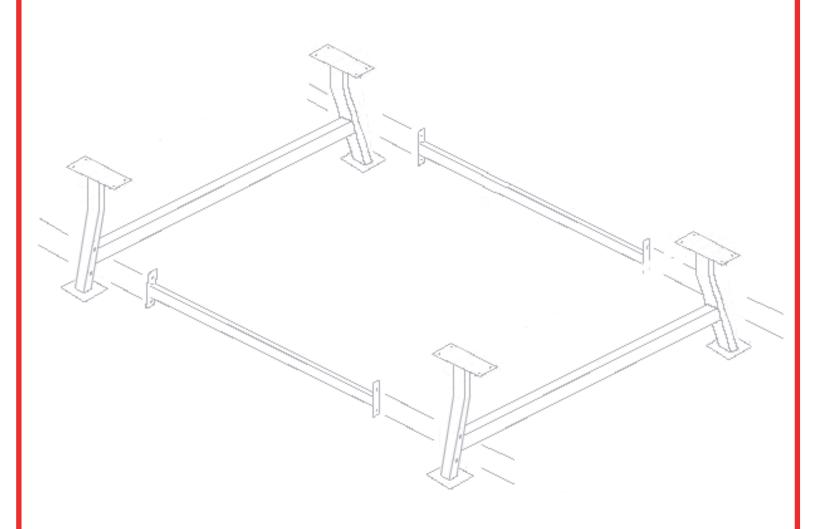
Fasten the two inch (2'') cross-members to the seven foot (7') main frames using eight (8) half inch by three and a half inch  $(1/2'' \times 3-1/2'')$  bolts, nuts and locks.
