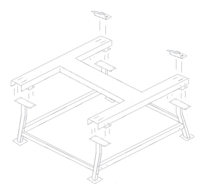
Mount the channel base frame to the main structure using sixteen (16) half inch by one and a half inch  $(1/2" \times 1-1/2")$  bolts, nuts and locks.
