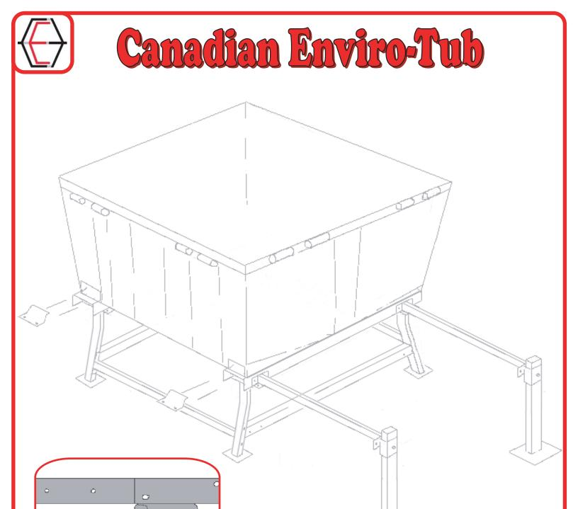
Place bottom half of the Enviro-Tub on the channel frame.
