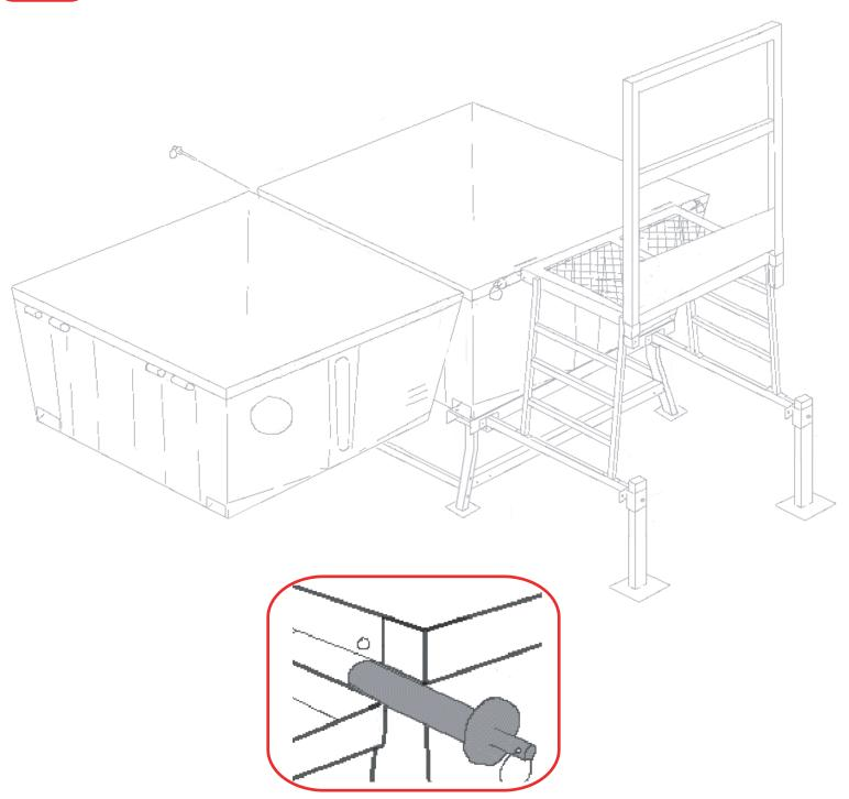
Connect the upper tub section to the lower tub section using two (2) hinge pins.
