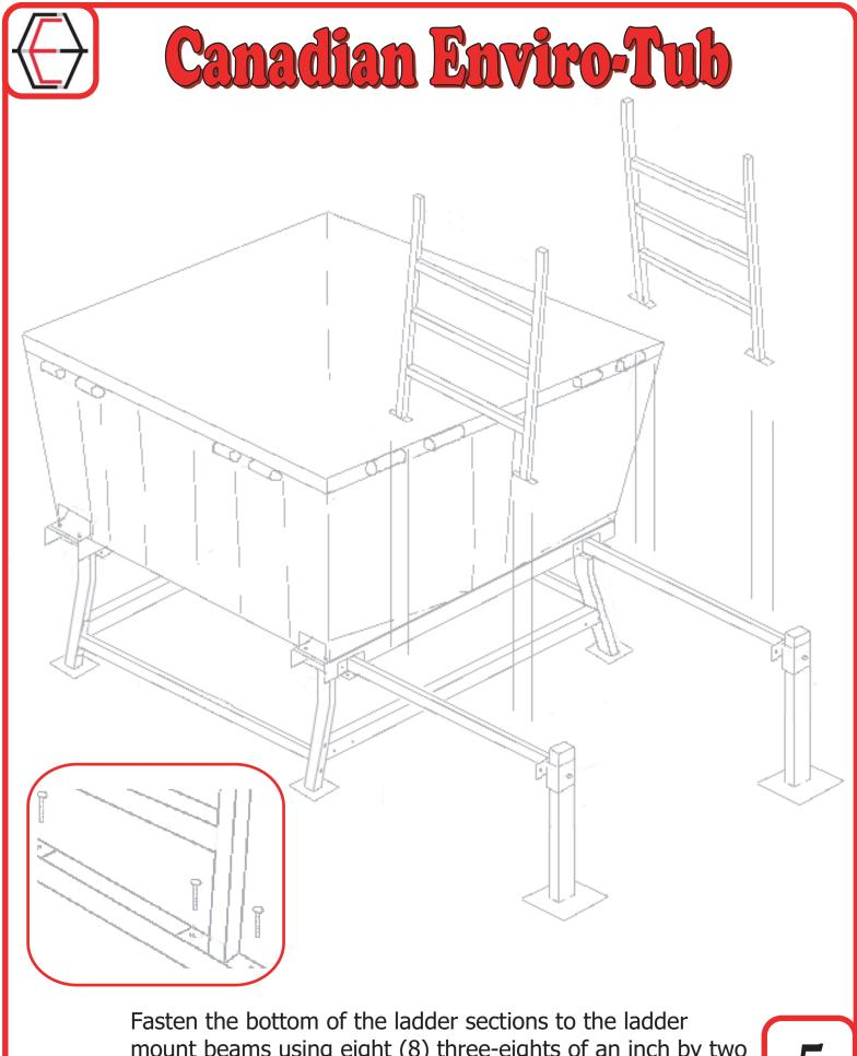
mount beams using eight (8) three-eights of an inch by two and a half inch  $(3/8" \times 2-1/2")$  bolts, nuts and locks.
