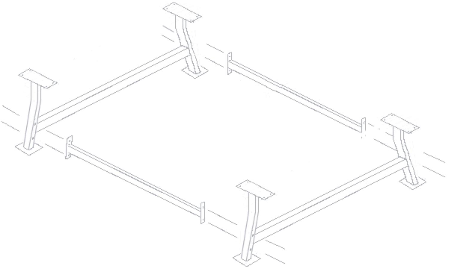
Fasten the two inch (2") cross-members to the seven foot (7') main frames using eight (8) half inch by three and a half inch (1/2" x 3-1/2") bolts, nuts and locks.
