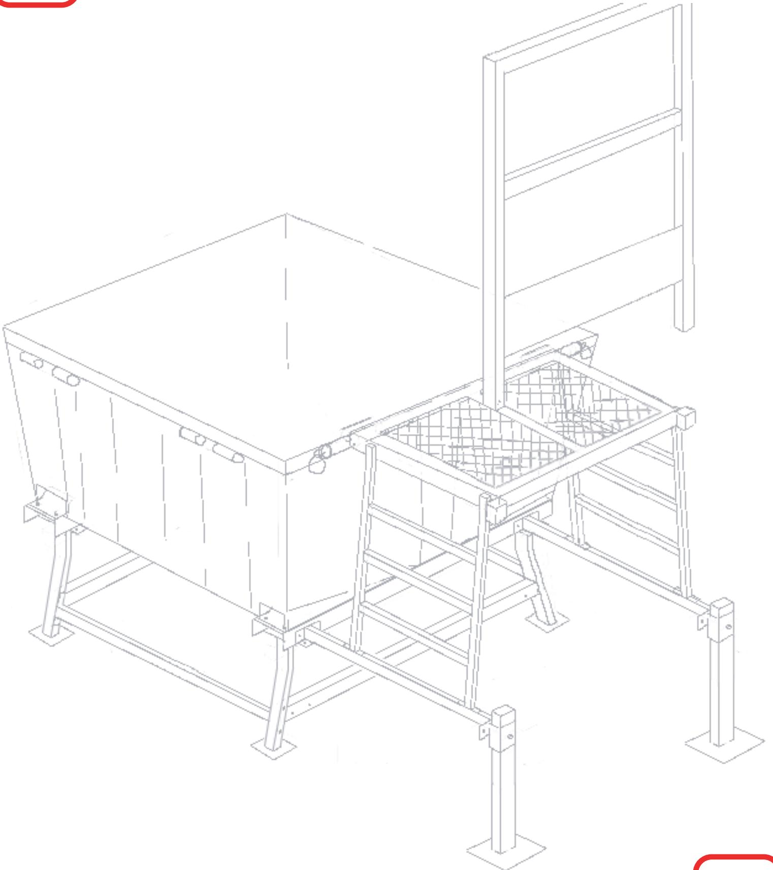
Insert the handrail into the platform handrail mount pockets and secure using two (2) safety pins.
