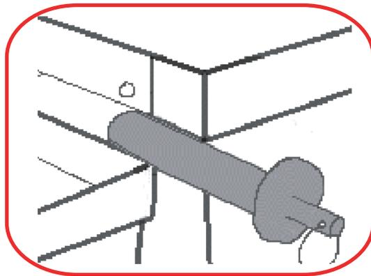
Connect the upper tub section to the lower tub section using two (2) hinge pins.
