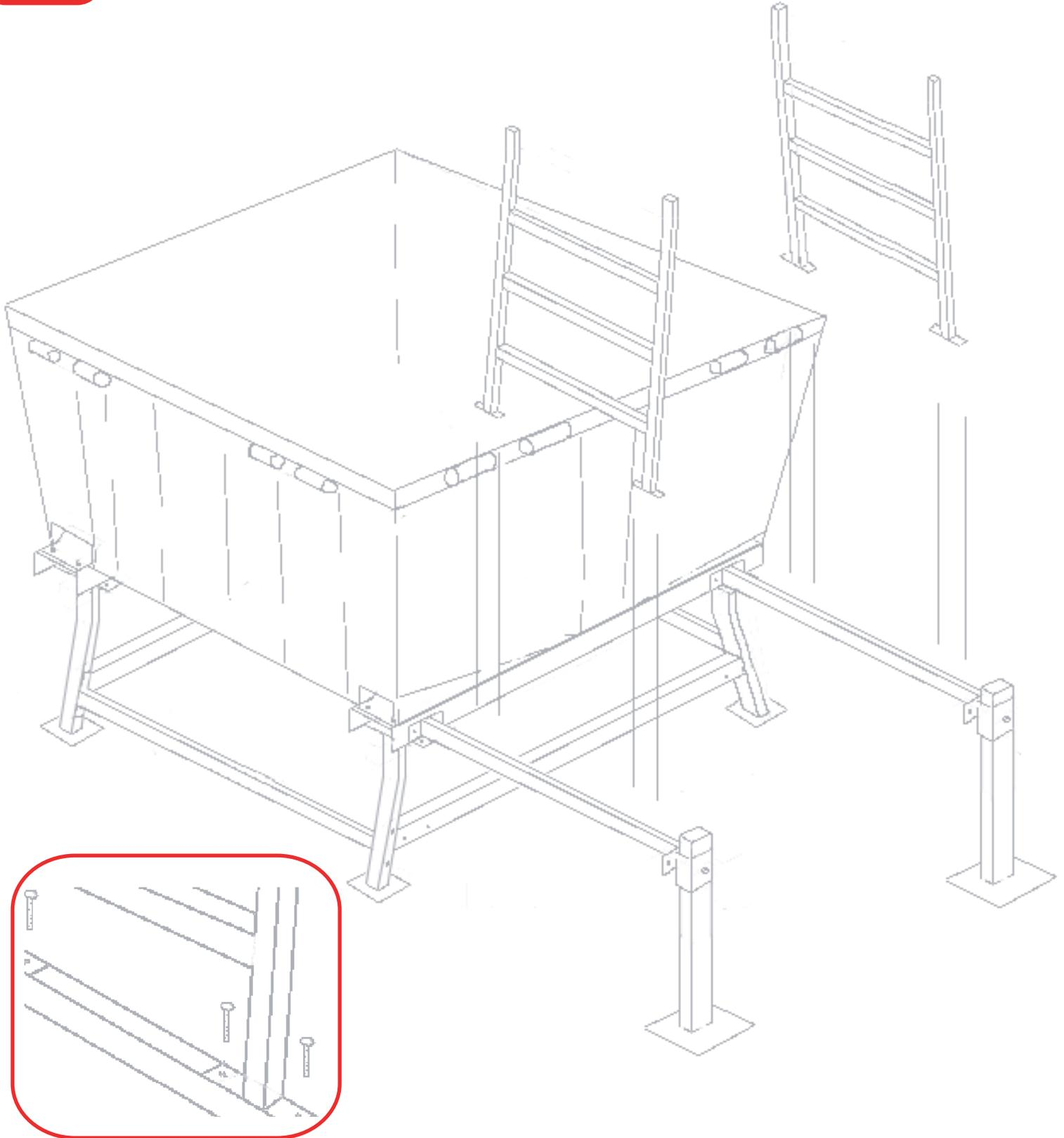
Fasten the bottom of the ladder sections to the ladder mount beams using eight (8) three-eighths of an inch by two and a half inch ( $3/8'' \times 2-1/2''$ ) bolts, nuts and locks.
