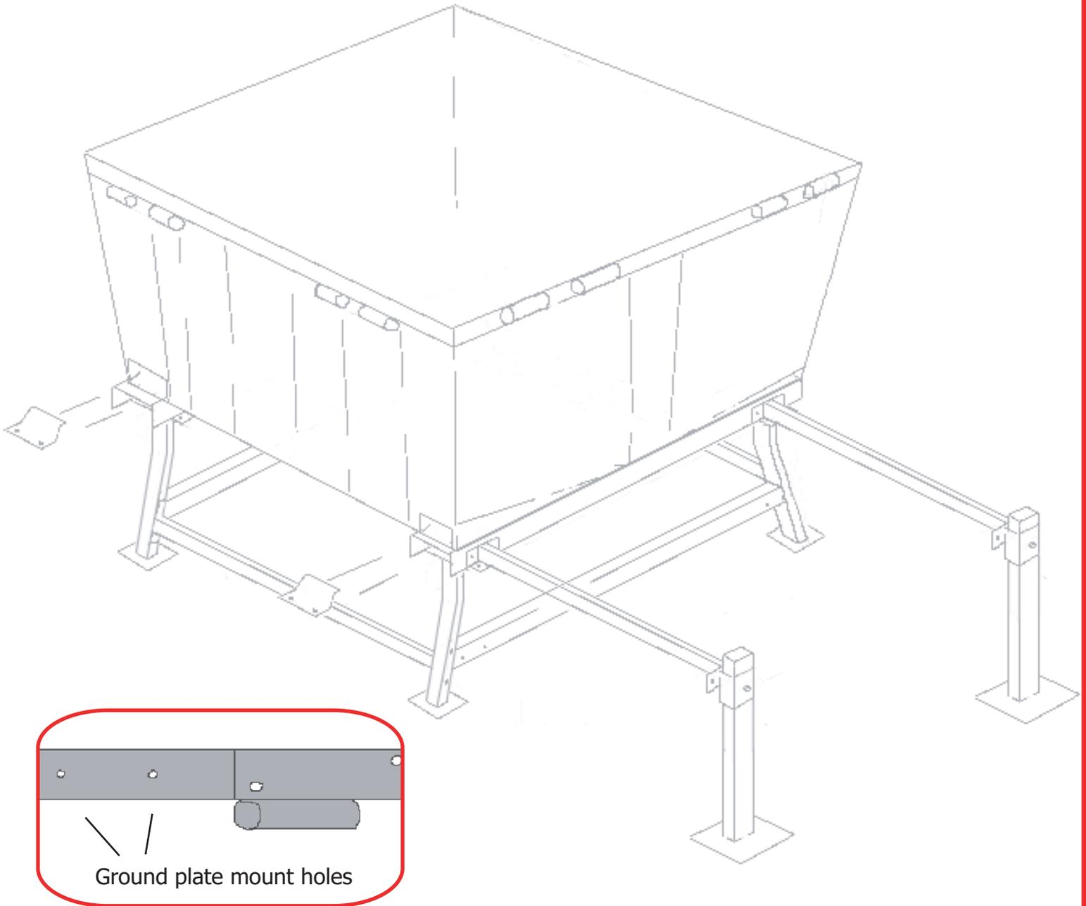
Place bottom half of the Enviro-Tub on the channel frame.
