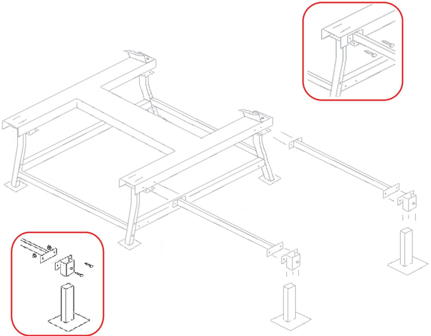
Fasten the ladder mount beams to the main frame cross beam using four (4) half inch by three and a half inch ( $1/2'' \times 3-1/2''$ ) bolts, nuts and locks.
