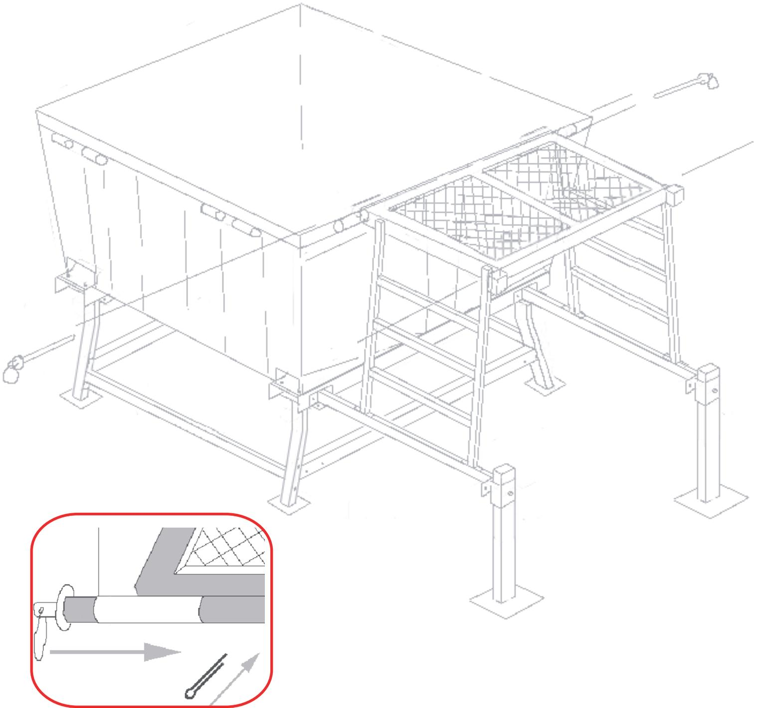
Insert the plate form hinge pins to secure platform to the tub. Making sure to insert safety pins.
